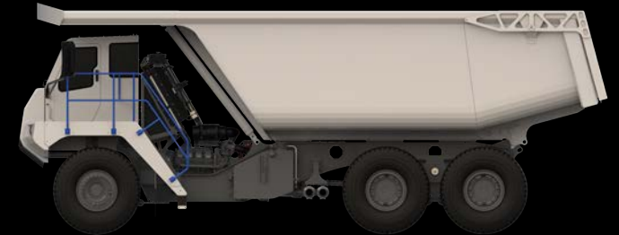
60 tonne, light material body up to 70 m 3 capacity suitable for coal and similar low density materials
