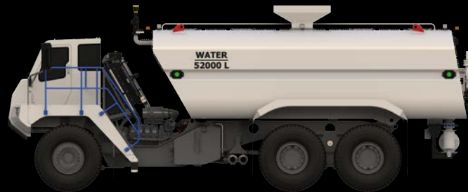
52,000 litre capacity flexible platform for fleet service requirements or haul road watering .
