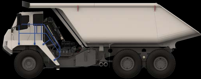
60 tonne, general purpose body suitable for overburden, hard rock and aggregates
